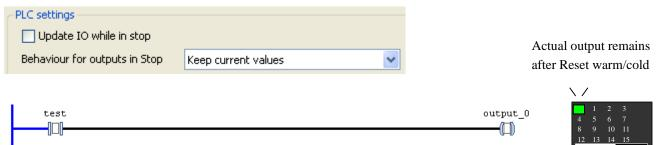
This is expected behaviour however, if this mismatching is to be avoided, change the setting of either "Update IO while in stop" or "Behaviour for outputs in Stop".
